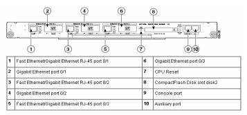
The three interfaces on the NPE-G1 consist of three Gigabit Interface Converter (GBIC) ports and three 10/100/1000 Fast Ethernet/Gigabit Ethernet ports. The rules for using these ports are:
